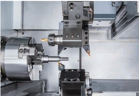
Upper & lower twin turrets synchronously work on spindle 1
