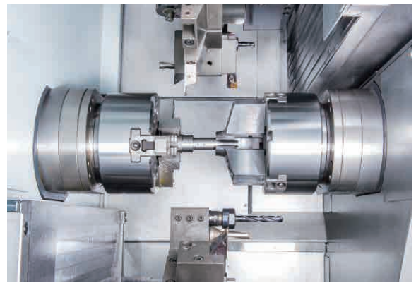
Twin spindles simultaneous part catching
